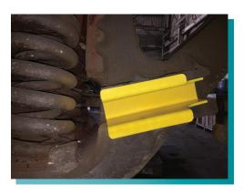
Brake beam shift accelerates flange wear on one wheel making wheelset unusable
