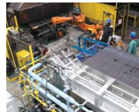
Steel bars are robotically sized, cut and precision tapered at both ends.
