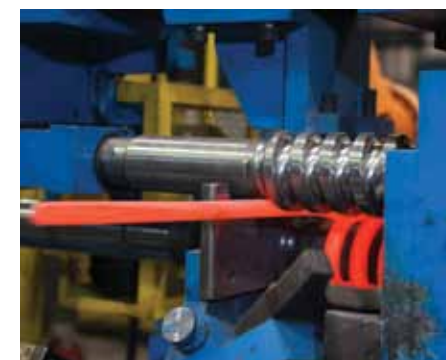
Easily changed coil dies allow for multiple spring sizes on the same assembly line.
